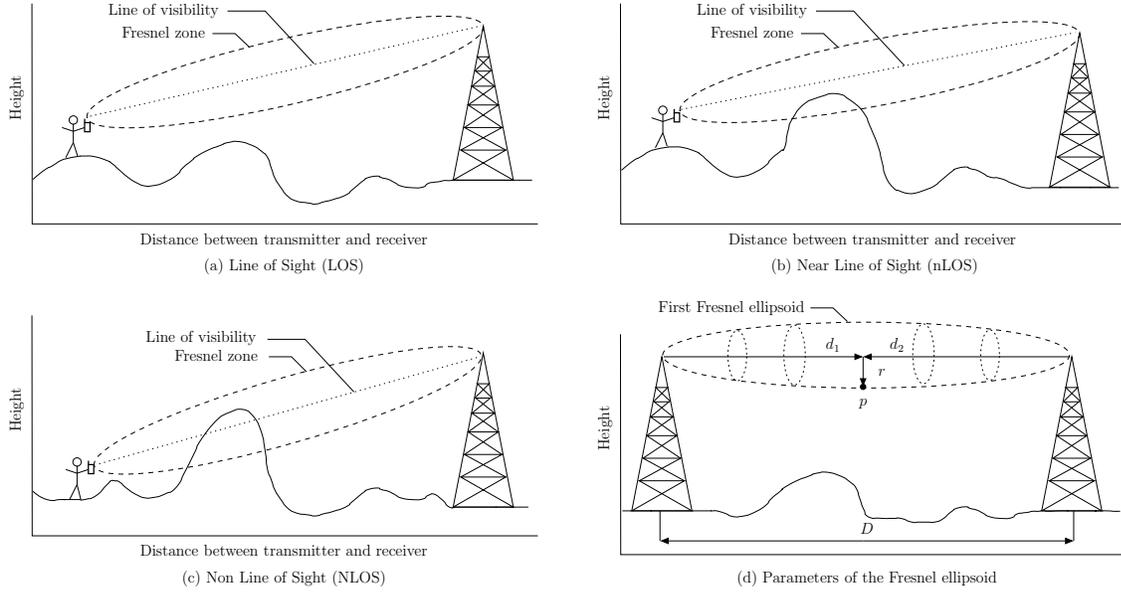
**Figure 1:** Various notions related to line of sight and the first Fresnel ellipsoid between a radio transmitter and receiver.
