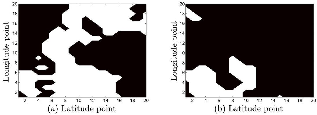
**Figure 3:** Viewshed of the area covered by a transmitter placed at (a) point (1,5) and (b) point (8,1).
